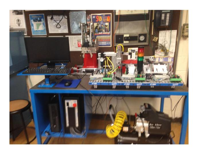
Attachment 2: Pegasus Robotic Arm and Three Station Programmable Logic Controllers (PLC's).
